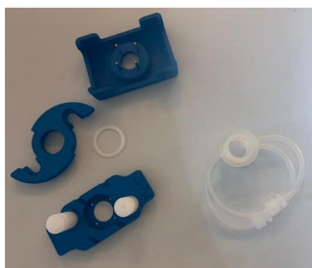
Microfluidic system for cell cultivation on transwells
